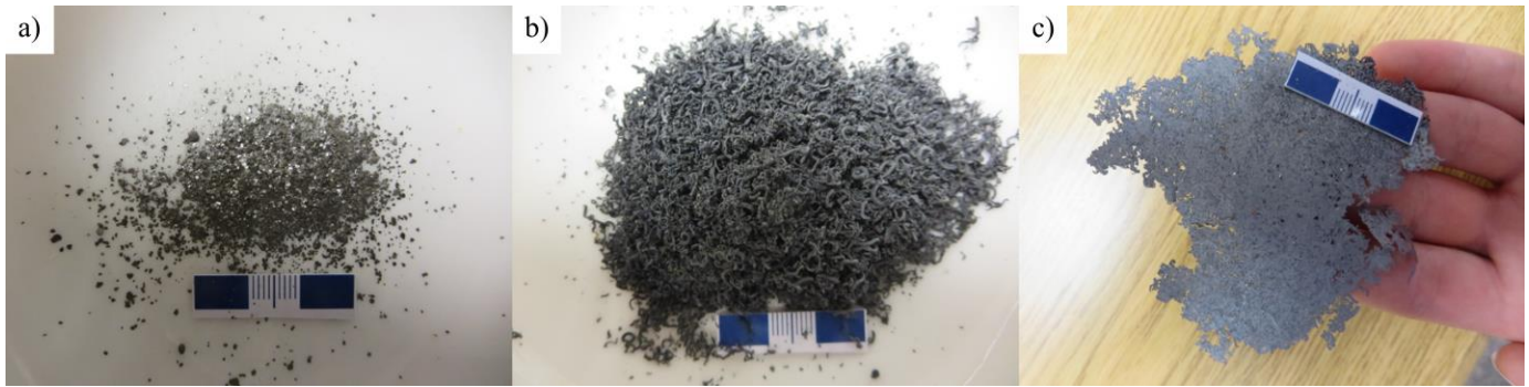
Figure 1: Manufacturing of Natural Graphite Sheet (NGS). a) flake graphite before exfoliation, b) after exfoliation, c) compressed exfoliated graphite. (Photographs reprinted from [7] with a permission from George Simandl)
